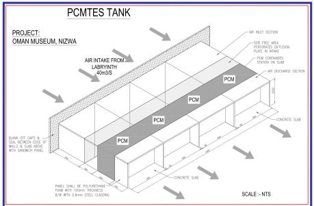
Each chamber 2.5m(8') (W) x 2.0m (61/2') (L) x 2.5m (8') (H) filled with 10 wide x 58 high FlatICE stack.
